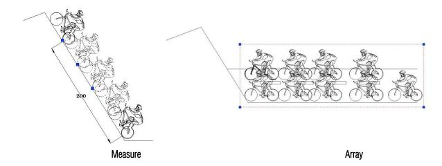
Layout By Path: Unlike common array function, LayoutByPath distributes object copies along a path (curve) with a variety of array options. Users can choose ra8ndom, division and measure options and array in different directions along the path.
