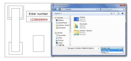
modified, it will be integrated into the specified block. It should be noticed that the imported file can't be attribute file exported by ATTOUT command, whereas the file format should be identical to that of ATTOUT command exporting.
