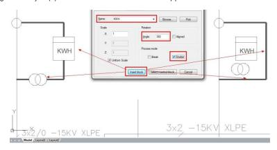
Replace Block with Another Block: In the current drawing, you can use one block to replace another one. Moreover, you can purge the unreferenced block when the operation is finished.
