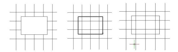
**Extended Offset:** This enhanced version of the OFFSET command offers several advantages over the standard command, including layer control, undo, and a multiple option.
