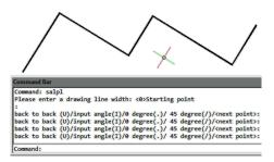
**Visual Extension:** Normally after extension, the extension effect will be displayed, but Visual Extension can display the effect in real time until you confirm the position.
