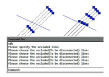
Control Break Width: This function is used to set break width for cross objects.
