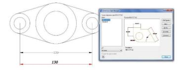
Reset Dim Text Value: Restore a measurement value to overridden or modified dimension text.
