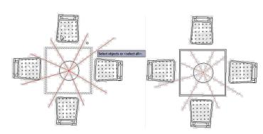
Extend to Nested Objects: Extends objects such as line segment, arc, polyline or ray to a block. Objects would be extended to a block as close as possible if they cannot intersect with each other.
