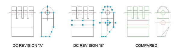
**Drawing Compare:** Drawing compare is an exclusive function in GstarCAD which is added according to the user's requirement.
