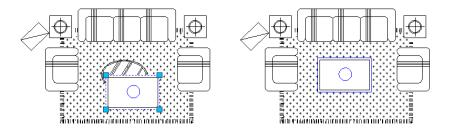
Breakline Symbol: Creates a polyline and inserts the breakline symbol. The options within this command are provided to control the relative size and appearance of the breakline symbol and an extension of the polyline beyond the selected start and end points.
